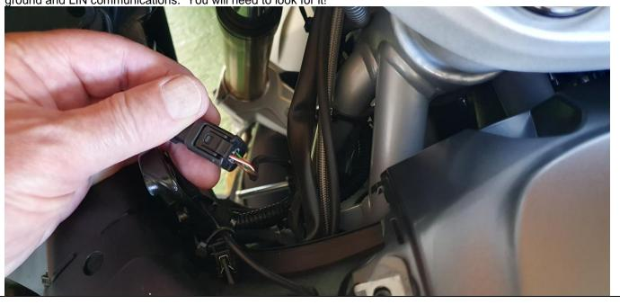
If you are connecting a GPS cradle / mount that is not from BMW, you likely do not have the 3x connector needed to plug into the GPS plug as noted above.
